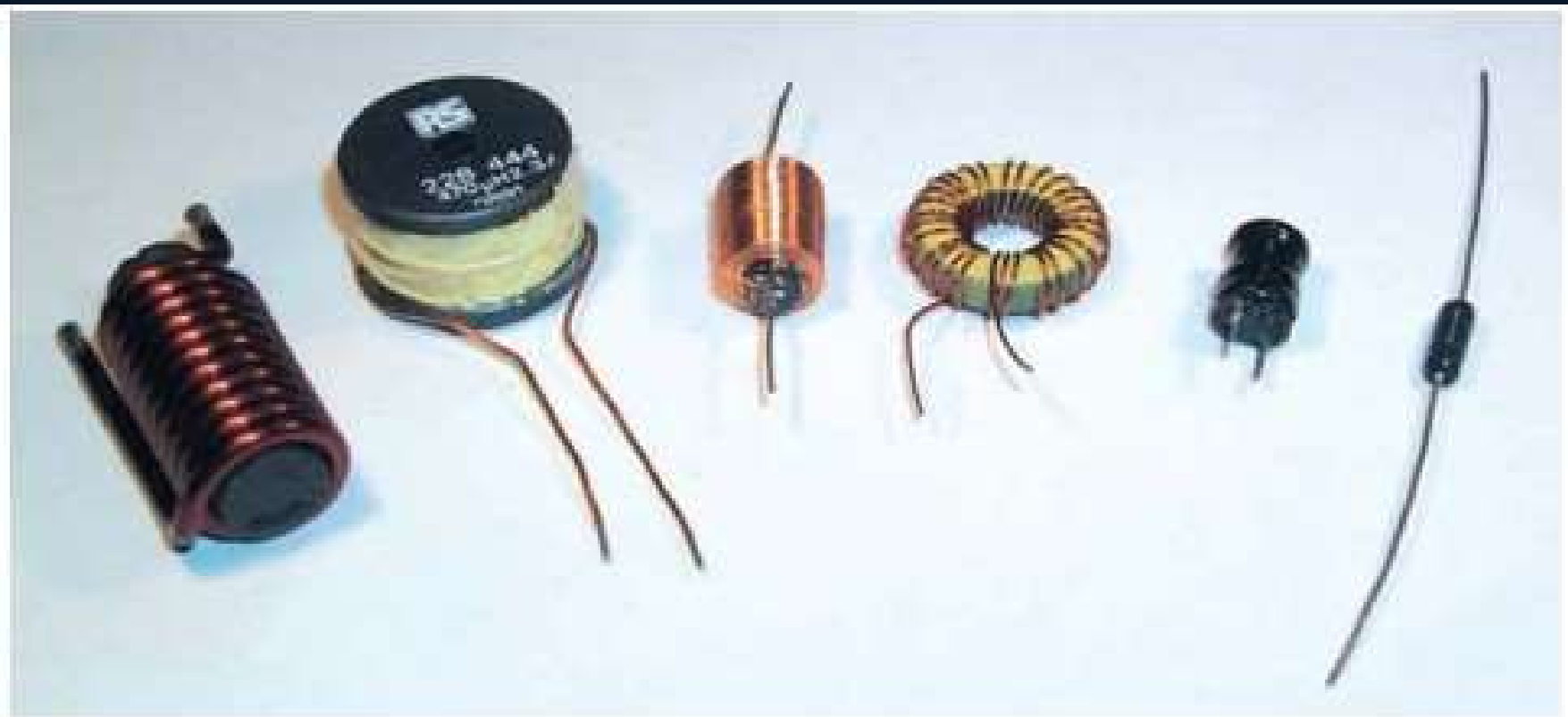
Various inductors with values ranging from 10\mu\text{H} to 1\text{mH} at current ratings from 100\text{mA} to 25\text{A}
